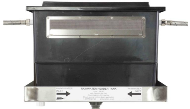
AB18T – Rainwater header with Type AB air gap. Supplied complete with stainless steel screened slot, wall bracket incorporating drip tray, two float valves and two inlet hoses with servicing valves.
