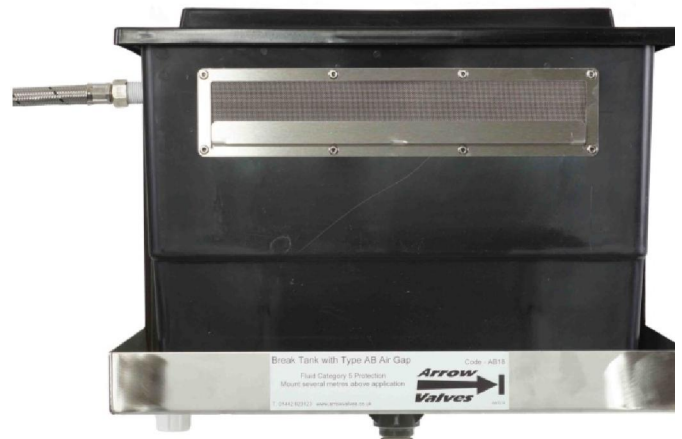
AB18 – Cistern with Type AB air gap. Supplied complete with stainless steel screened slot, wall bracket incorporating drip tray, float valve and inlet hose with servicing valve.
