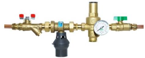
CA15C297PRV - Filling valve assembly comprising of – inlet Servicing Valve c/w serviceable strainer, CA Device, Pressure Reducing Valve (PRV) and Servicing (isolating) Valve. Normally set to 1.5 bar
