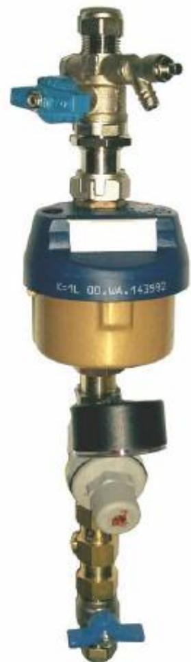
Branch Valve & Meter Assembly (model BRPMV). Typical assembly manufactured by Arrow Valves. Supply to apartments - isolating, Double Check, PRV, meter and isolating
