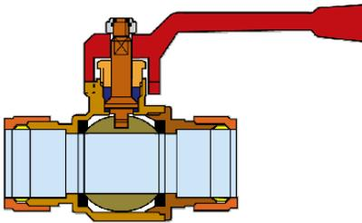
BV209 section - showing serviceable PTFE spindle seal
