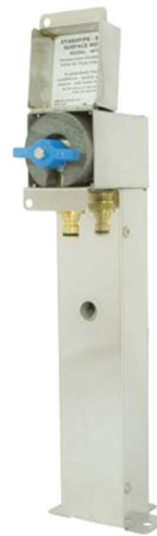
Model SPTG Low level Standpipe with Double Check Valve for Fluid Category 3 protection. Flange enables mounting to flat surface – concrete or flat roof for window cleaning and roof garden watering
