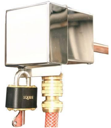
Model HUTB15 (shown with optional padlock and hose connector socket). Polished stainless steel box. The rear entry copper tube passes through the wall (use sleeve or insulation) and is cut to length after installation. For surface run external supply pipe, use model HUTBS, HUTBT or HUTG – see page 3
