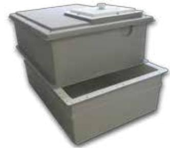
The tank will arrive with the sections assembled with one fixing in each corner of the joint flange to allow transportation to site. Remove the corner fixings to allow positioning of the tank.
