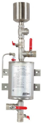
Dosing Pot (model DP) Supplied with five full-bore spherical servicing valves, safety check valve, funnel and mounting brackets
