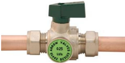
Automatic Flow Limiting (AFL) Valve. Servicing Valve with flow limiting cartridge. Arrow Valves AFLs have a lever and colour coded-coded identity disc indicating the flow rate of the cartridge inside
