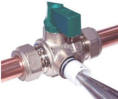
There are 8 colour-coded AFL cartridges that are fit into valve in-situ. Cartridge fits into centre of ball via side port – no need to isolate or drain supply . Pliers can be used to remove cartridge. A cartridge can be fitted or changed in less than a minute
