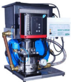
"Boost-A-Break®" Break tank and pump set with Type AB air gap (model BTAB) for Fluid Category 5. Flush WCs or urinals without additional backflow protection. Supplied as complete unit
