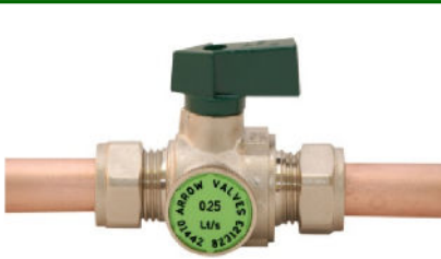
Automatic Flow Limiting (AFL) Valve. Servicing Valve with flow limiting cartridge. Arrow Valves AFLs have a lever and colour coded identity disc indicating the flow rate of the cartridge inside
