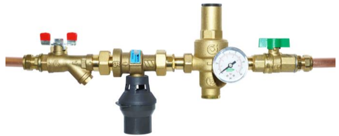
CA15C297PRV - Filling valve assembly comprising of – inlet servicing valve c/w serviceable strainer, CA device, Pressure Reducing Valve (PRV) and servicing (isolating) valve
