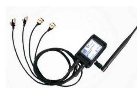
The temperature monitoring unit incorporates an aerial, and two ports to which cables connect, and are then attached at the other end to the pipework or outlet.
