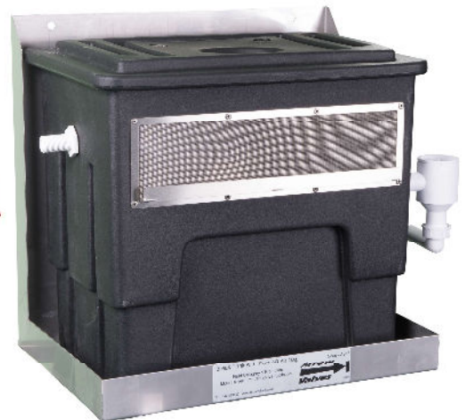
AB18 – Cistern with Type AB air gap. Supplied complete with stainless steel screened slot, wall bracket incorporating drip tray, float valve and inlet hose with servicing valve.
