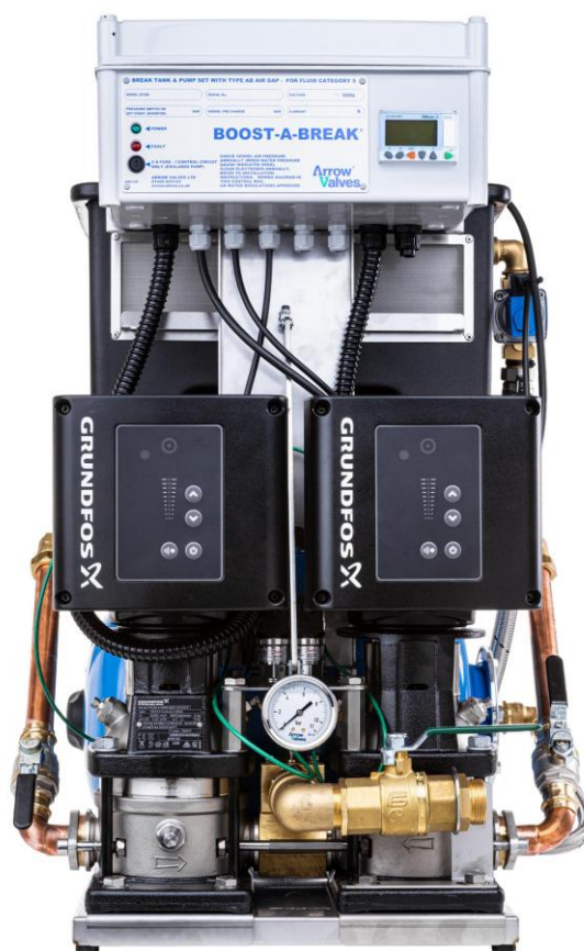
Model 3-10A Dual Pump - Duty Assist. Pumps alternate daily to prevent stagnation. Flow output up to 2.4 Lt/s
